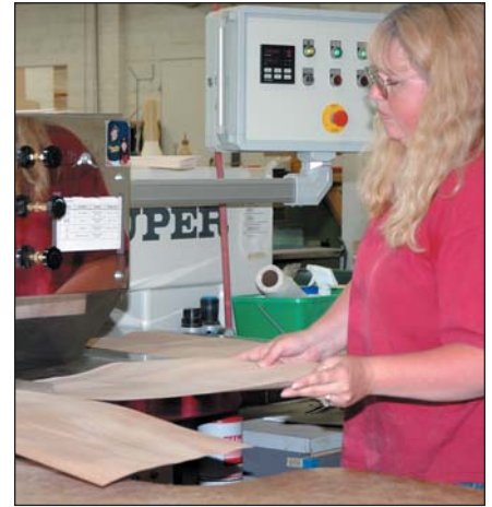
Putting the pieces together — Nancy Gardner puts together the individual veneer components in sequence. When she finishes she signs off on it. Every employee has to assess the work at every stage and sign off on it.
