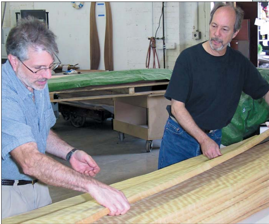
Dedicated to veneer — This part of the 10,000-square-foot shop is dedicated to processing veneer components into architectural veneer panels. Beyond this room is an area where curved panels and panels that require more preparation are handled. Adjacent to the processing areas is a storage area.
