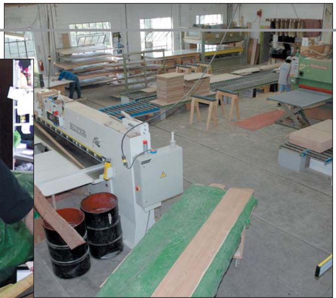
Dedicated to veneer — This part of the 10,000-square-foot shop is dedicated to processing veneer components into architectural veneer panels. Beyond this room is an area where curved panels and panels that require more preparation are handled. Adjacent to the processing areas is a storage area.
