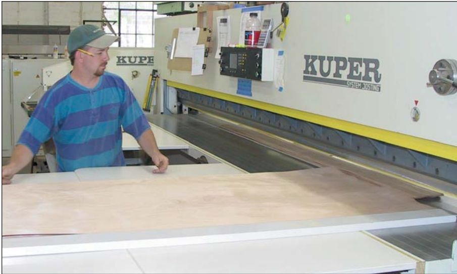
Clipping flitches — Each veneer flitch is clipped sequentially and in a balanced way to the desired size on the Kuper guillotine by Chris Strother. He numbers each panel's worth of veneer.
